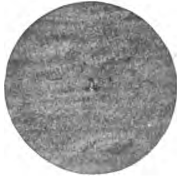
Fig. 14. Pearlite Area predominating; Carbon, 0.90 Per Cent
